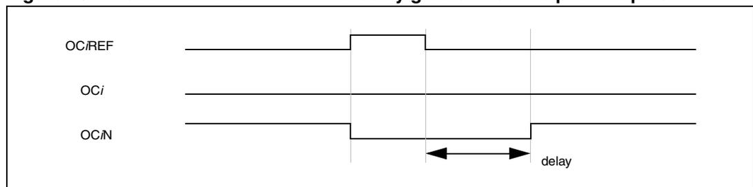
The deadtime delay is the same for each of the channels and is programmable with the DTG bits in the  $TIM1\_DTR$  register. Refer to [Section 17.7.31: Deadtime register \(TIM1\\_DTR\) on page 212](#) for delay calculation.
