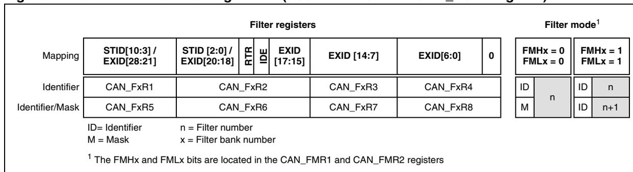
**Figure 148. 16-bit filter bank configuration (FSCx bits = 0b10 in CAN\_FCRx register)**
