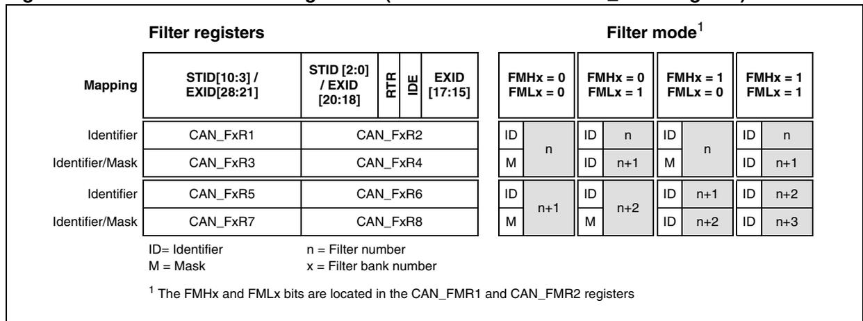
Figure 149. 16/8-bit filter bank configuration (FSCx bits = 0b01 in CAN\_FCRx register)
