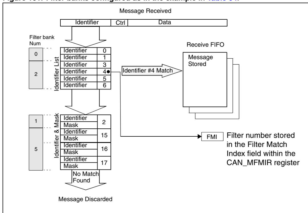
The example above shows the filtering principle of the beCAN. On reception of a message, the identifier is compared first with the filters configured in identifier list mode. If there is a match, the message is stored in the FIFO and the index of the matching filter is stored in the Filter Match Index. As shown in the example, the identifier matches with Identifier #4 thus the message content and FMI 4 is stored in the FIFO.
