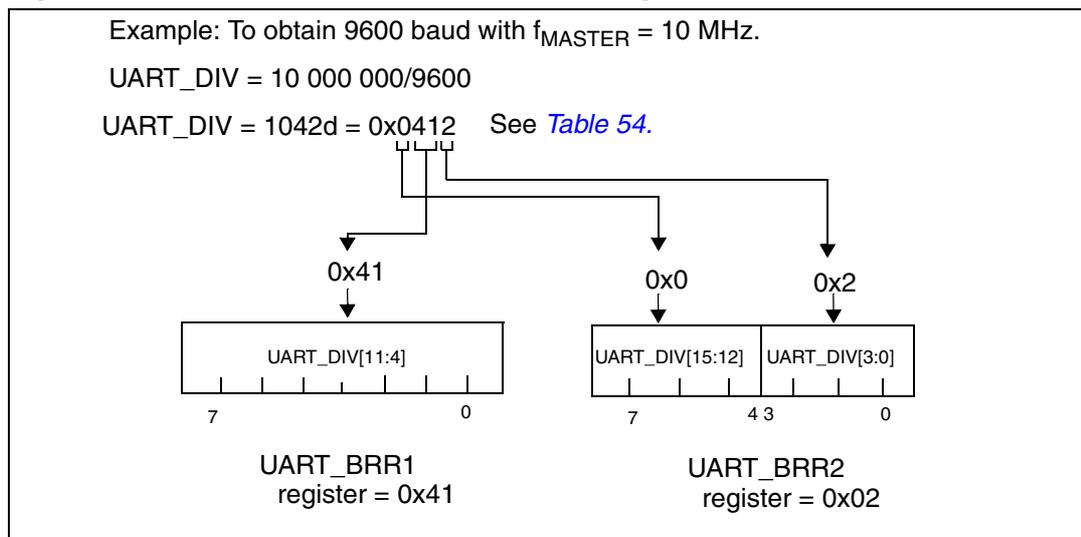
*Note:* The Baud Counters will be updated with the new value of the Baud Registers after a write to BRR1. Hence the Baud Register value should not be changed during a transaction. The BRR2 should be programmed before BRR1.
