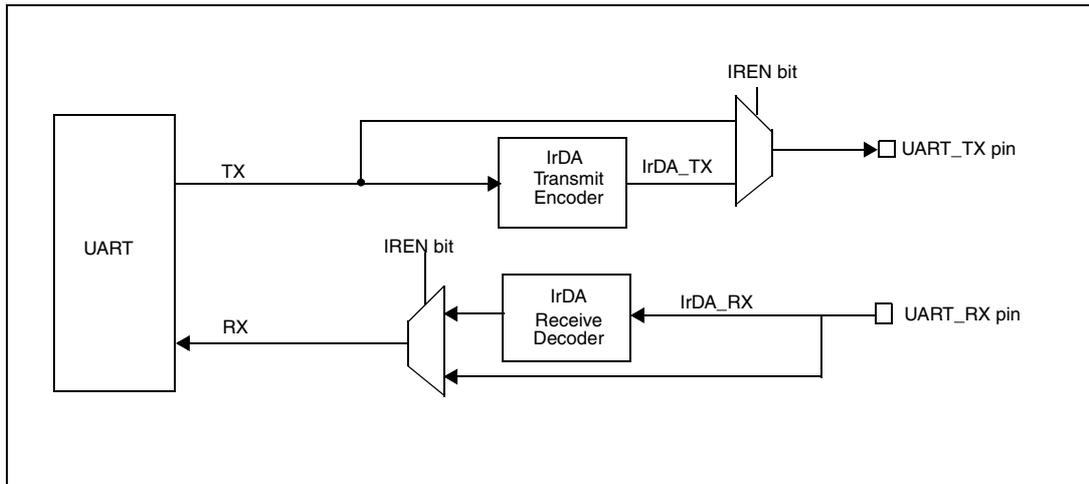
Figure 128. IrDA data modulation (3/16) - normal mode
