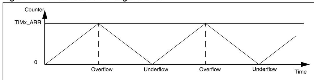
If the timer has a repetition counter (as in TIM1), the UEV is generated after up and down counting and repeated for the number of times programmed in the repetition counter register (TIM1\_RCR). Otherwise, the UEV is generated at each counter overflow and at each counter underflow.
