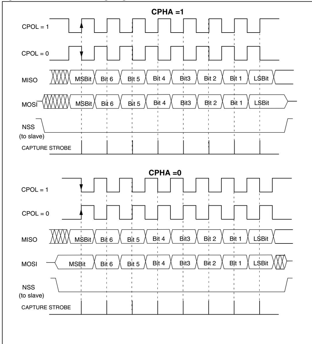
1. These timings are shown with the LSBFIRST bit reset in the SPI\_CR1 register.
