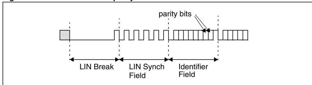
The bits involved are the two MSB positions (7th and 8th bits) of the identifier character. The check is performed as specified by the LIN specification:
