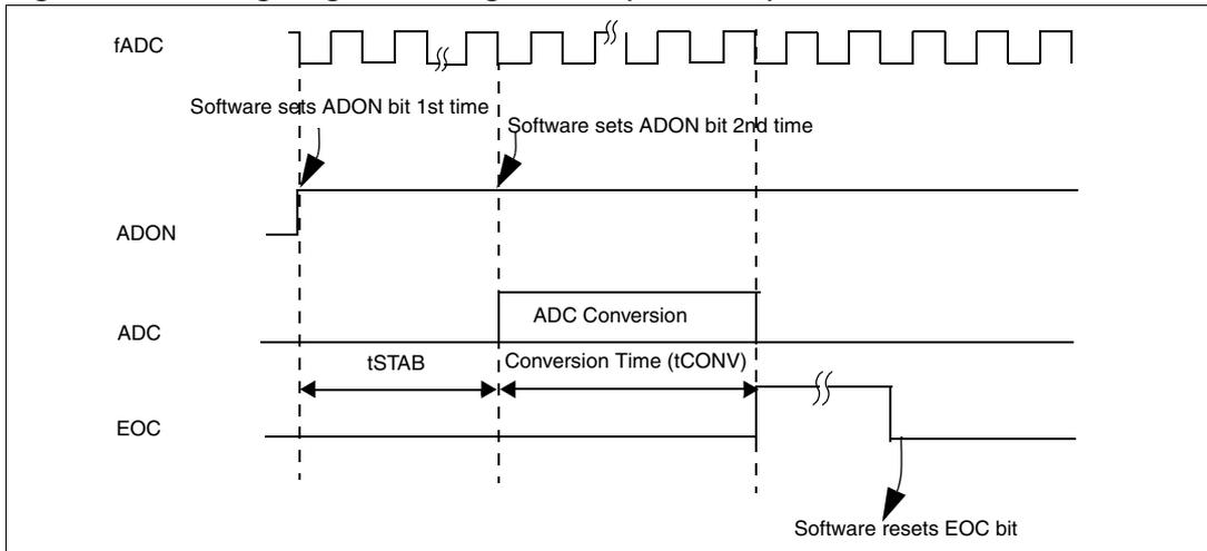
**Figure 162. Timing diagram in continuous mode (CONT = 1)**
