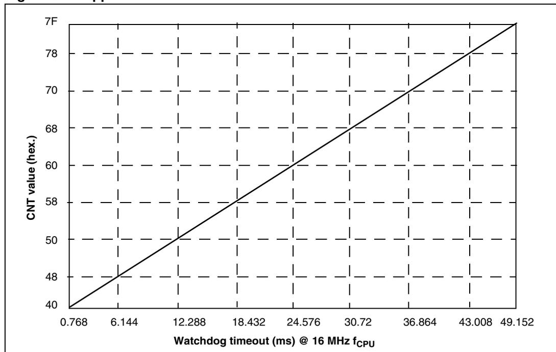
Figure 30. Window watchdog timing diagram
