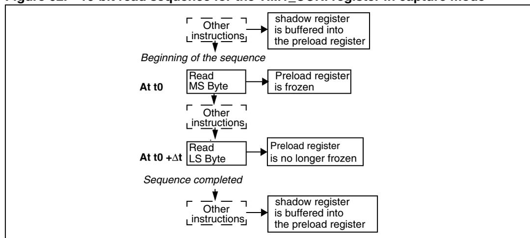
[Figure 62](#) shows the sequence for reading the  $CCRi$  registers in the 16-bit timers. This buffered value remains unchanged until the 16-bit read sequence is completed.
