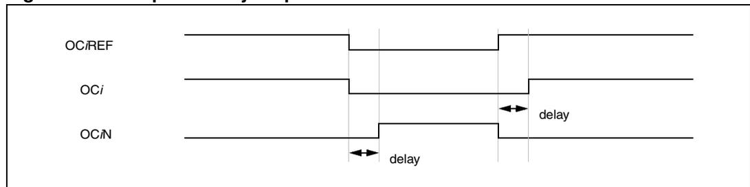
**Figure 74. Deadtime waveforms with a delay greater than the negative pulse**
