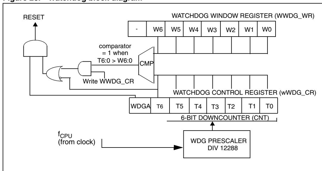
The application program must write in the WWDG\_CR register at regular intervals during normal operation to prevent an MCU reset. This operation must occur only when the counter value is lower than the window register value. The value to be stored in the WWDG\_CR register must be between 0xFF and 0xC0 (see [Figure 29](#)):
