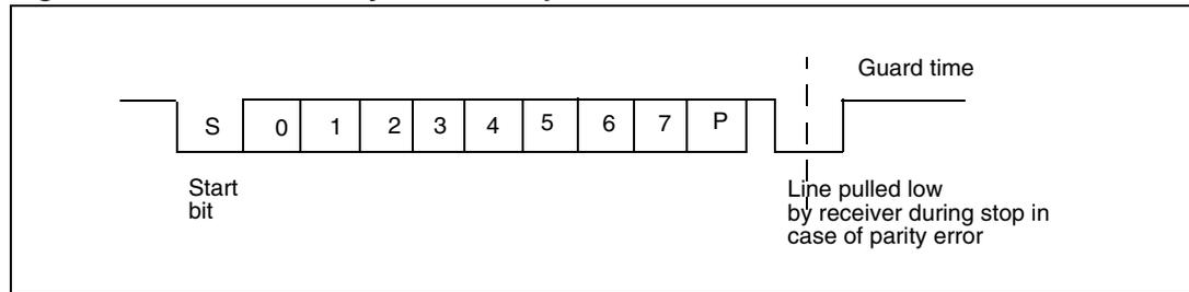
When connected to a smartcard, the UART\_TX output drives a bidirectional line that is also driven by the smartcard.
