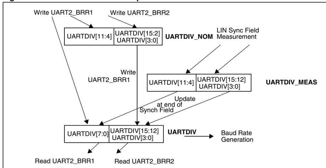
Figure 136. UARTDIV read / write operations when LDUM = 1
