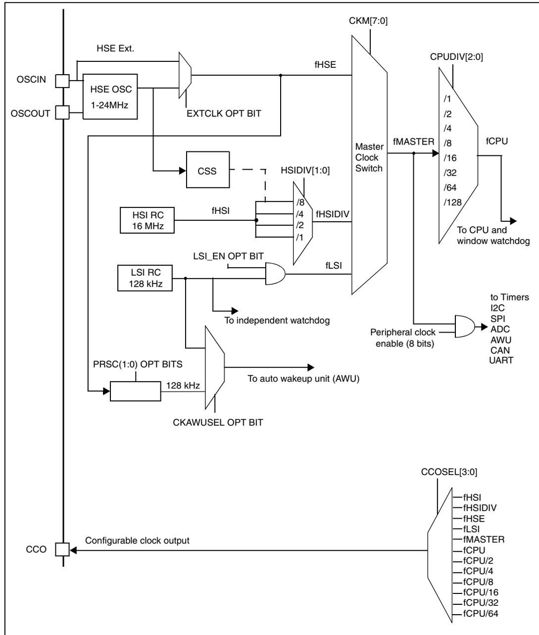
1. Legend: HSE = High speed external clock signal; HSI = High speed internal clock signal; LSI = Low Speed internal clock signal.
