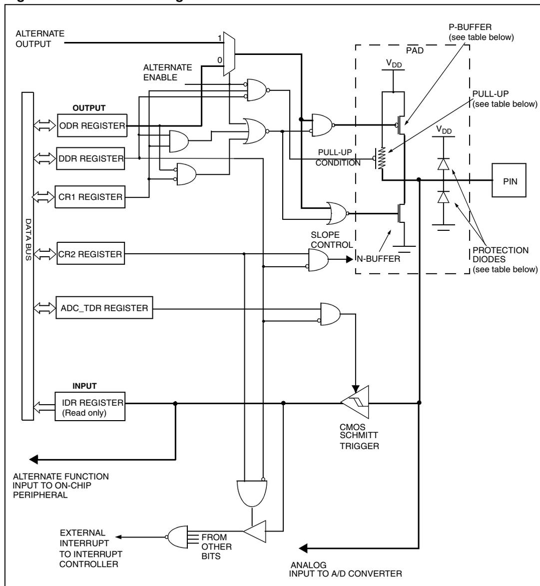
Note: The output stage is disabled when the analog input is selected.
