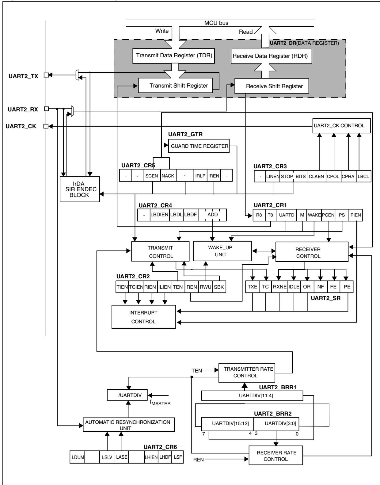
Figure 112. UART3 block diagram
