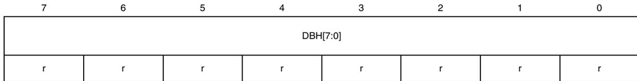
**Note:** *Data buffer registers are not available for ADC2. The data buffer size and base address are device dependent and are specified in the corresponding datasheet. Note that the data buffer registers and the other ADC registers have different base addresses.*
