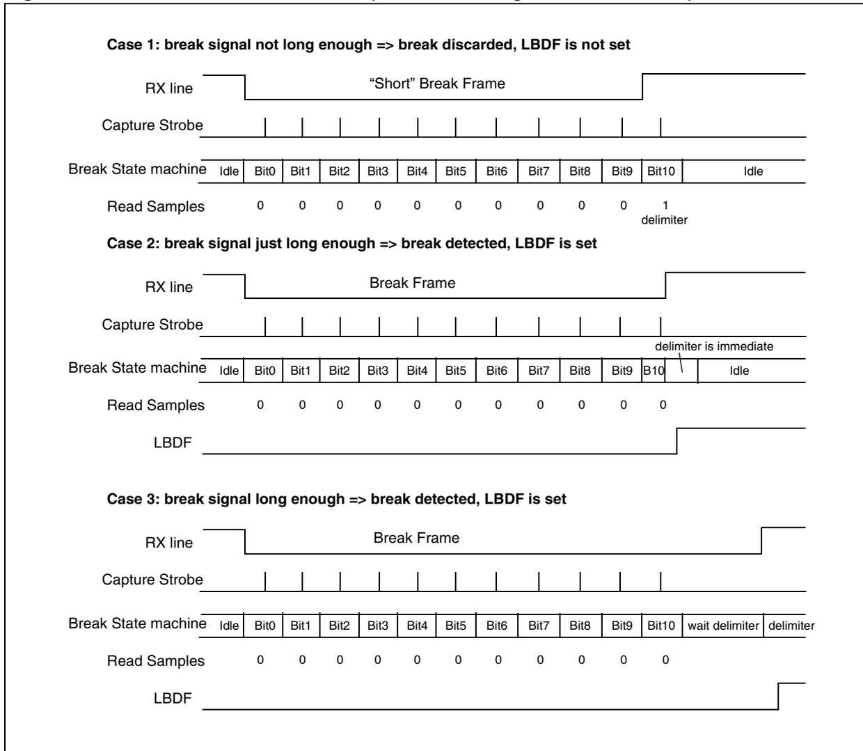
**Figure 130. Break detection in LIN mode vs framing error detection**
