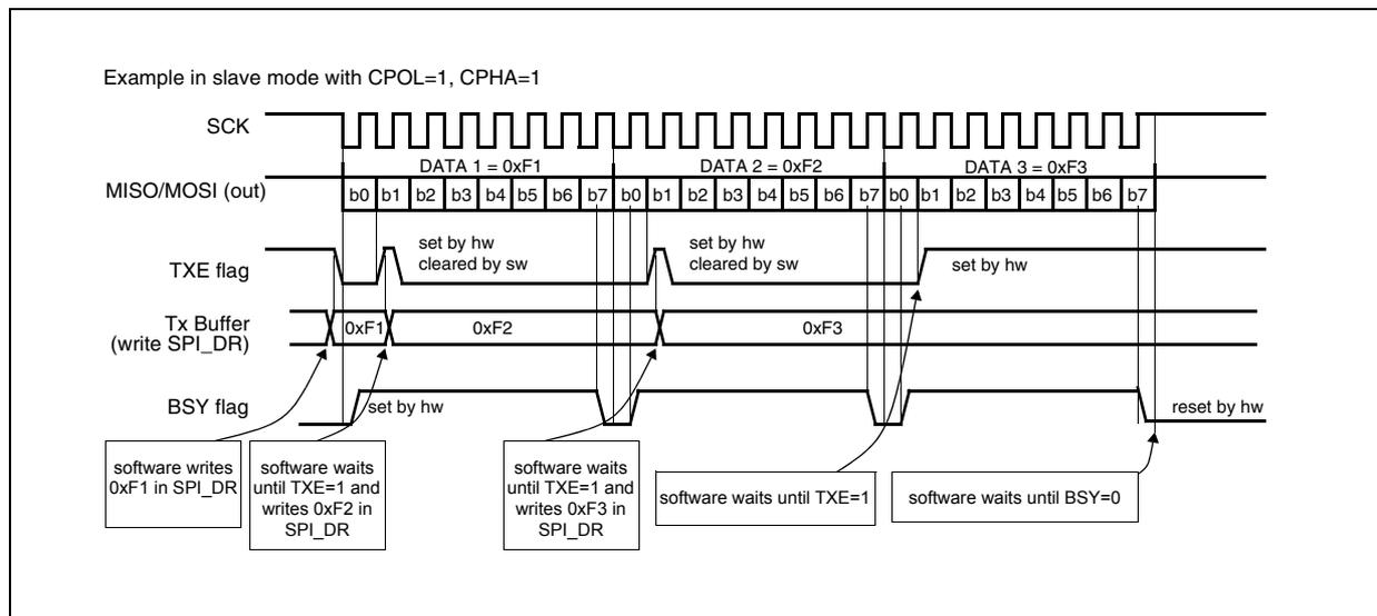
**Bidirectional transmit procedure (BDM = 1 and BDOE = 1)**
