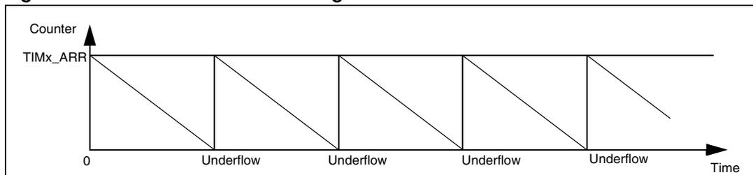
An update event can also be generated by setting the UG bit in the TIM1\_EGR register (by software or by using the clock/trigger mode controller).
