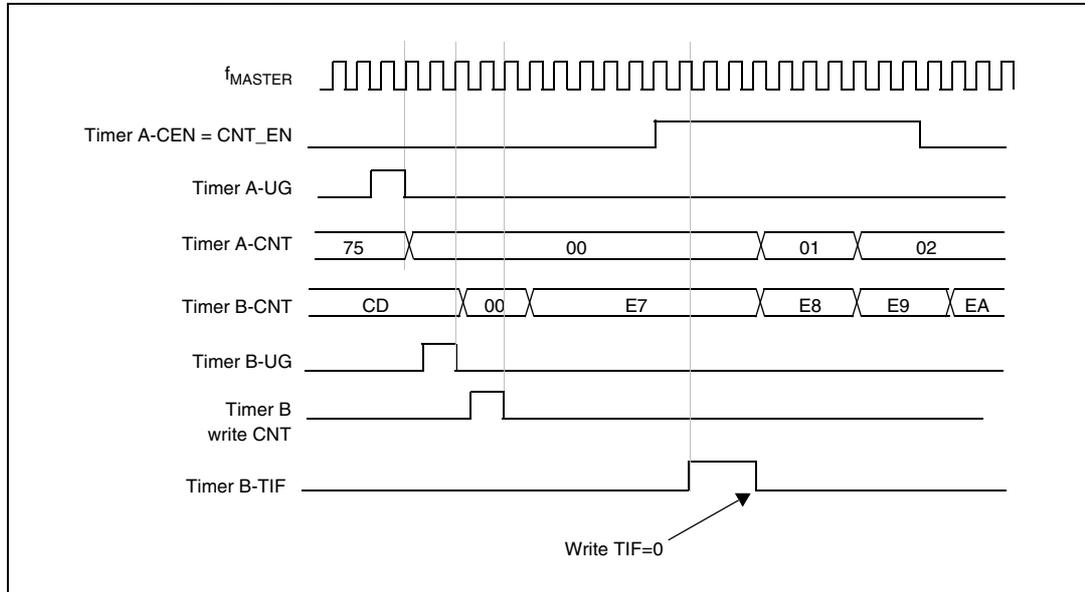
**Starting 2 timers synchronously in response to an external trigger****Example**
