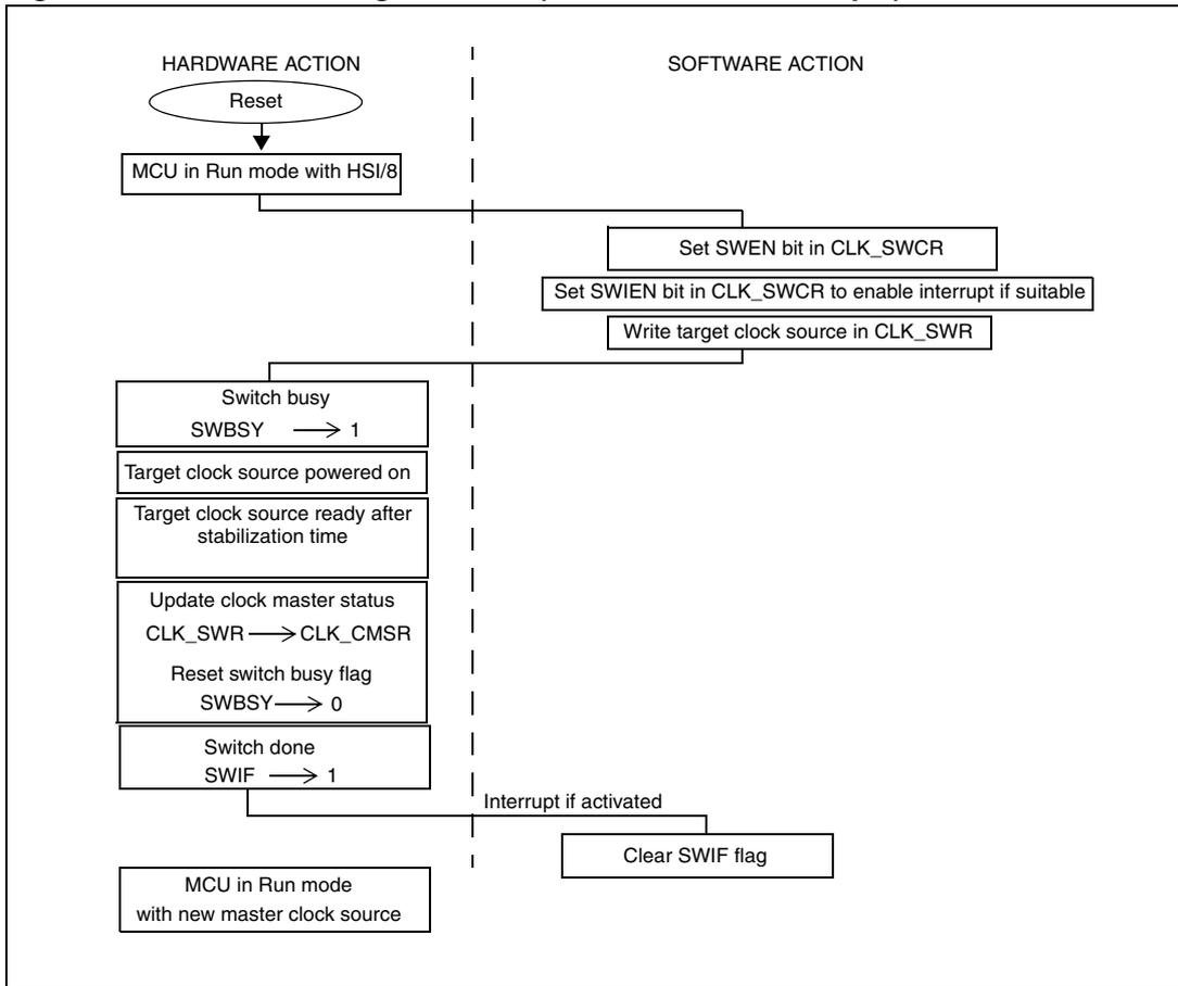
Figure 23. Clock switching flowchart (manual mode example)
