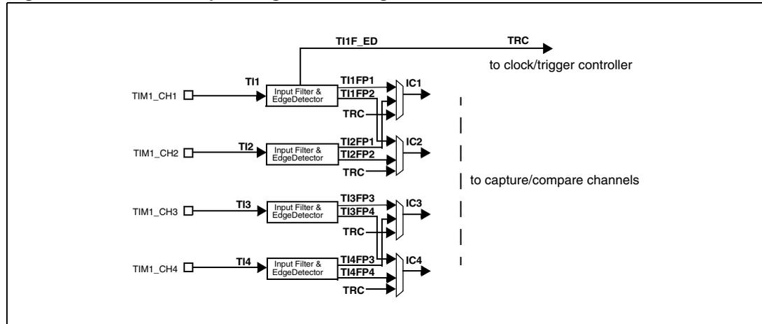
Figure 64 shows how the input stage samples the corresponding TI/ input to generate a filtered signal TI/F. Then, an edge detector with polarity selection, generates a signal (TI/FPn) which can be used as trigger input by the clock/trigger controller or as the capture command. The signal is prescaled before entering the capture register (IC/PS).
