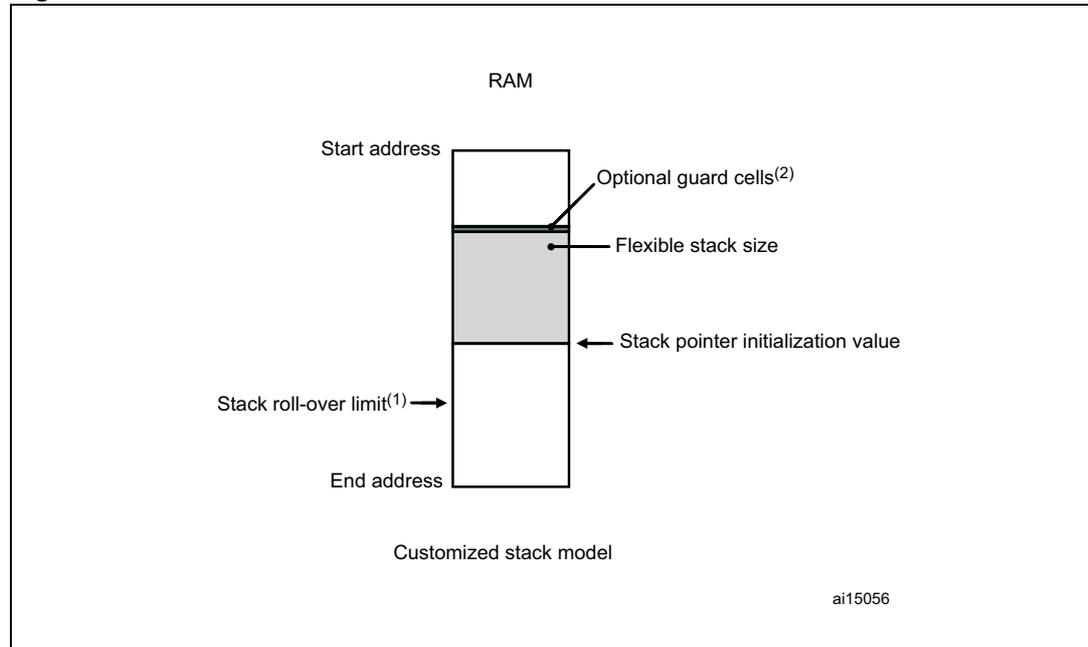
1. The stack roll-over limit is not implemented on all devices.
