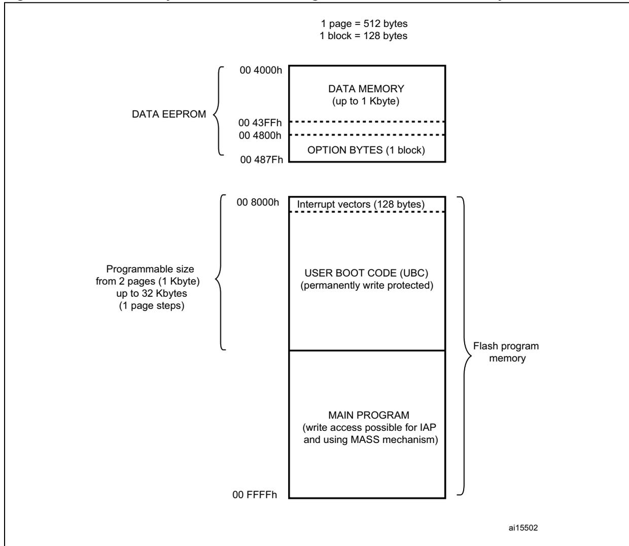
1. The memory mapping is given for the STM8A devices featuring 32 Kbytes of Flash program memory and 1 Kbytes of SRAM.
