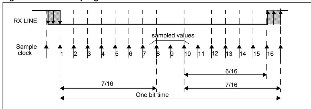
*Note:* The sample clock frequency is 16x baud rate.
