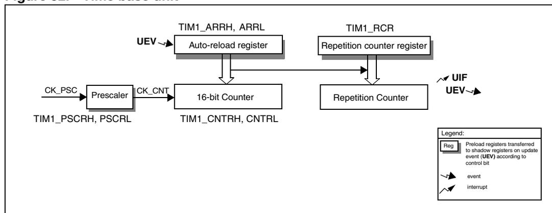
The 16-bit counter, the prescaler, the auto-reload register and the repetition counter register can be written or read by software.
