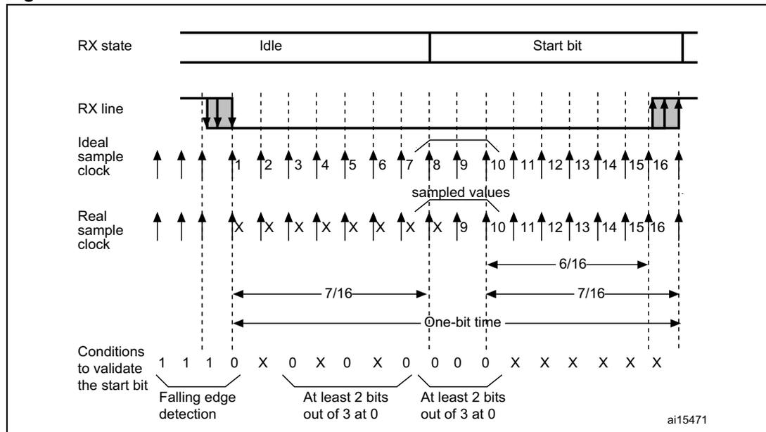
*Note:* If the sequence is not complete, the start bit detection aborts and the receiver returns to the idle state (no flag is set), where it waits for a falling edge.
