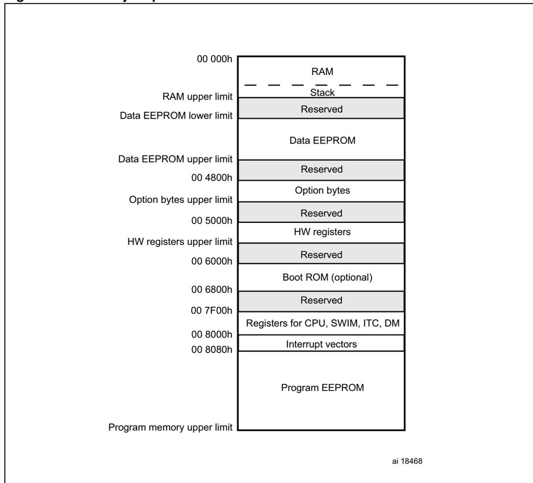
The RAM upper limit, data EEPROM upper and lower limit, Option Byte upper limit, hardware (HW) registers upper limit, and the program memory upper limit are specific to the device configuration. Please refer to the datasheets for quantitative information.
