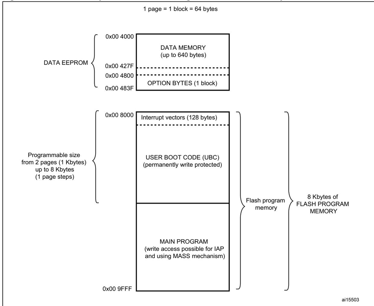
Figure 7. Flash memory and data EEPROM organization on medium density STM8S and STM8A
