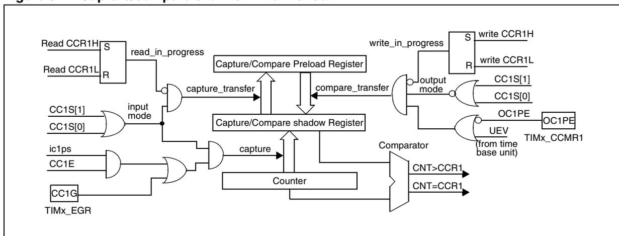
The capture/compare block is made of one preload register and one shadow register. Write and read always access the preload register. In capture mode, captures are made in the shadow register, which is copied into the preload register. In compare mode, the content of the preload register is copied into the shadow register which is compared to the counter.
