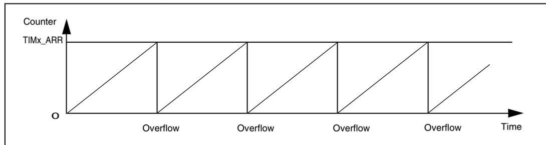
An update event can also be generated by setting the UG bit in the TIM1\_EGR register (either by software or by using the trigger controller).
