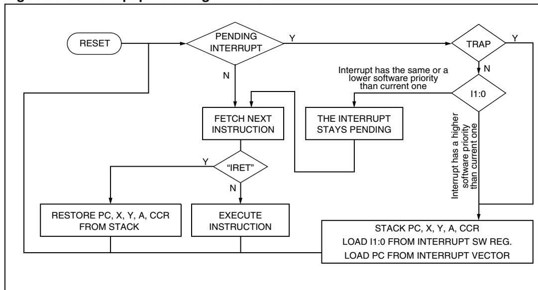
**Caution:** If the interrupt mask bits I0 and I1 are set within an interrupt service routine (ISR) with the instruction SIM, removal of the interrupt mask with RIM causes the software priority to be set to level 0.
