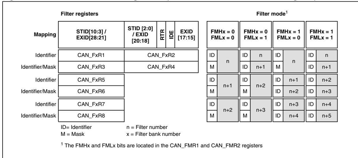
Figure 150. 8-bit filter bank configuration (FSCx bits = 0b00 in CAN\_FCRx register)
